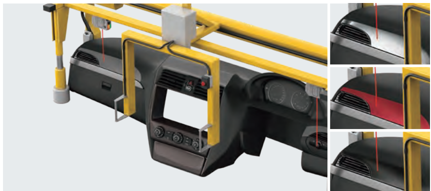
Presence detection of interior decoration parts
