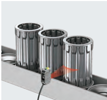
Presence detection of needle bearings
