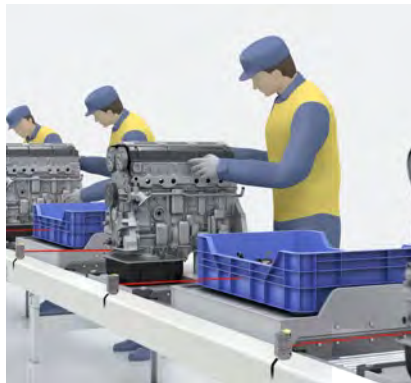
Presence detection of pallets
