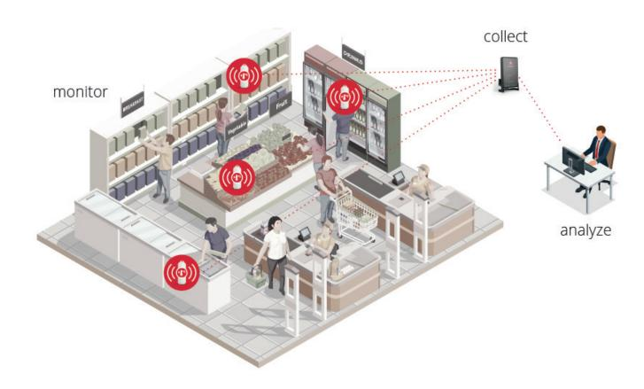
THE SENSORS SEND THE DATA TO THE BASE STATION & RESPONSIBLE PERSONELL CAN ANALYZE DATA ON PC, TABLET OR PHONE
