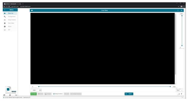
**Figure 14:** View Live page. This shows the live view while no acquisition is running. Mouse cursor position is indicated in "x" and "y" text fields.
