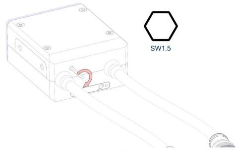
Figure 8: Adjusting the focus
