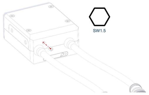
Figure 7: Removing the hexagon socket set screw
