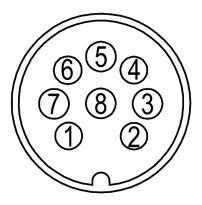
Figure 2: Pin assignment M12 connector
