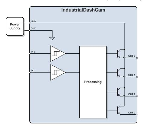
Figure 3: Simplified digital I/O circuit
