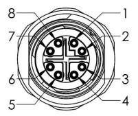
Figure 5: Pin assignment M12 connector
