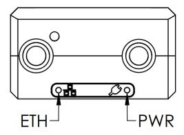
Figure 6: VisionDevice status LEDs
