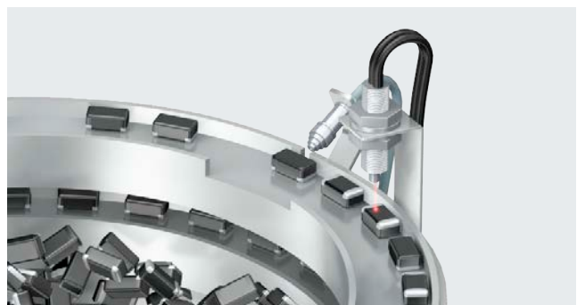
Air blower output during chip's front/rear detection
